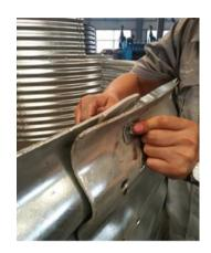
Seal Gap by Silicone Sealant
